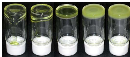
Fig. 2 Optical images of five blends of AI-10 : X ( X = 0.5, 0.75, 1, 2, and 3 ). The blends were displayed in the order of X value from left to right. Gels were not formed at small amount of PEI for X = 0.5 or 0.75 . At the optimum amount of PEI ( X = 1 ), however, homogeneous and transparent gels were formed. A gel state had been kept up to large amount of PEI ( X = 2, 3 ), though the appearance of cloudiness or turbidity is evident.
